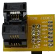
Figure 14 – Various socket adapters are available
